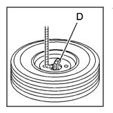
Tilt the retainer at the end of the cable and pull it through the wheel opening. Pull the tire out from under the vehicle.
